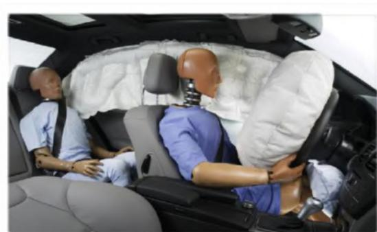
Different safety systems and working principles were also discussed. Students now know about the working of an airbag and the seat belt setup. This lecture helped the students understand how safety is important and how the manufacturer concentrates on these. Cross-section of airbag systems were presented and passed on to each student to have a better understanding of the system. The overall feedback of the lecture was good.
