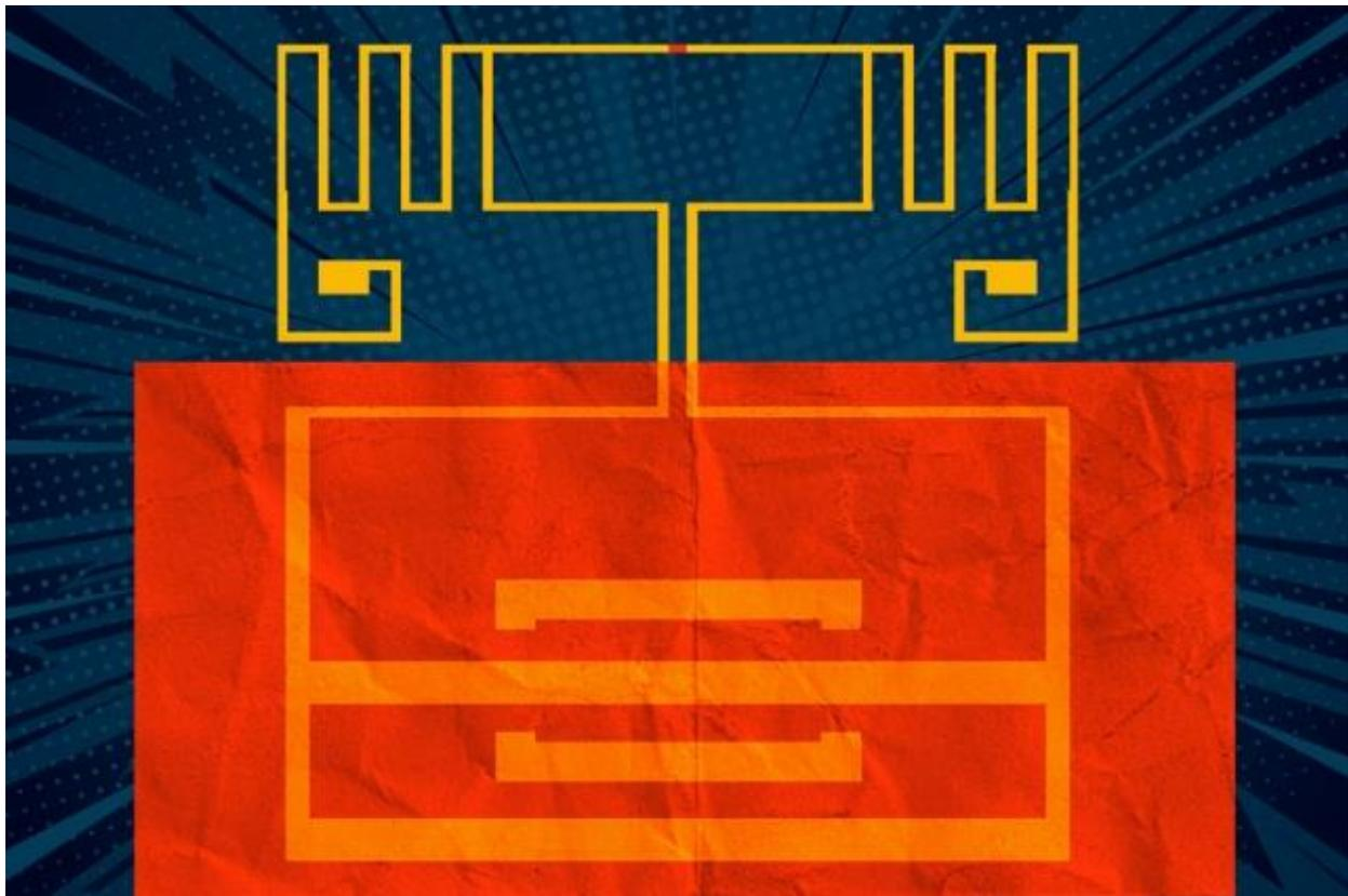
Devices that convert AC electromagnetic waves into DC electricity are known as “rectennas.” The researchers demonstrate a new kind of rectenna, described in a study appearing in *Nature* today, that uses a flexible radio-frequency (RF) antenna that captures electromagnetic waves – including those carrying Wi-Fi – as AC waveforms.
