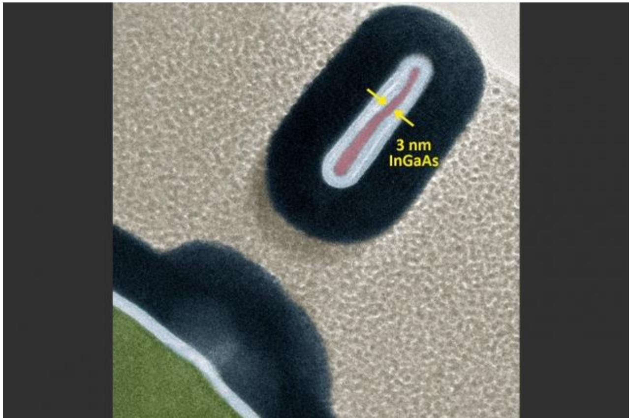
As described in a paper presented at this week's IEEE International Electron Devices Meeting, the researchers modified a recently invented chemical-etching technique, called thermal atomic level etching (thermal ALE), to enable precision modification of semiconductor materials at the atomic level. Using that technique, the researchers fabricated 3-D transistors that are as narrow as 2.5 nanometers and more efficient than their commercial counterparts.
